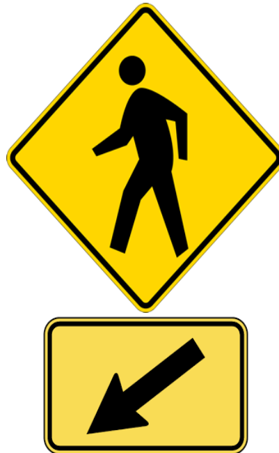
Pedestrian Crossing (W11-2) Warning Sign with Diagonal Downward Pointing Arrow (W16-7P)
